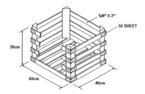
Figure 1: Crates used for storage & transport
