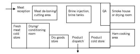
Figure 2: Layout of a meat processing room
