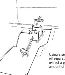
Using a sequence of oil separators will extract a greater amount of oil.
