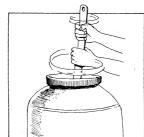
The fermentation lock consists of a cork with a hole in the centre through which passes a 5mm diameter plastic tube. This must end up in the glass, which contains a small spoonful of bisulphate in half a glass of water.
