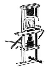
Figure 4: Oil press with a hydraulic jack
