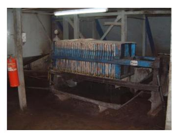
Figure 8: Typical filter press. Photo: Tony Swetman
