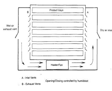
Figure 4: Schematic diagram of a cross flow cabinet
