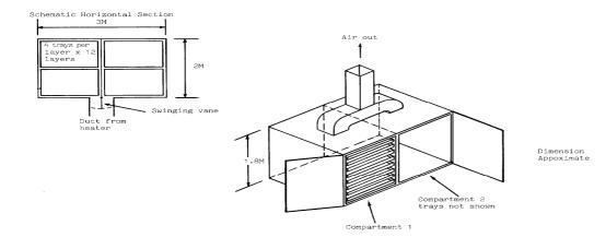
Figure 2: A typical double chamber batch dryer
