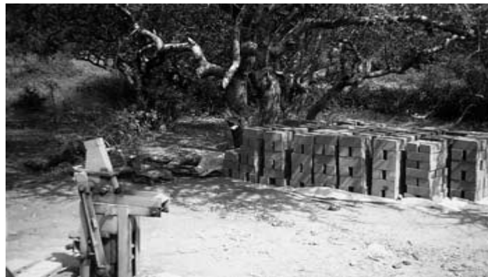
Stabilised soil block machine and stack of blocks curing in the shade of a tree. Photo: Practical Action / Theo Schilderman.
