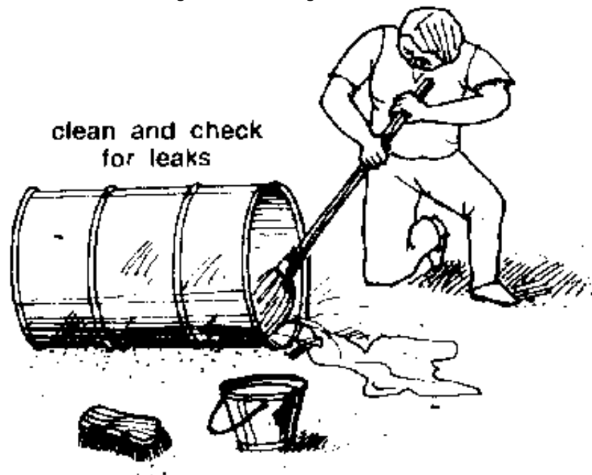
Clean and check for leaks
