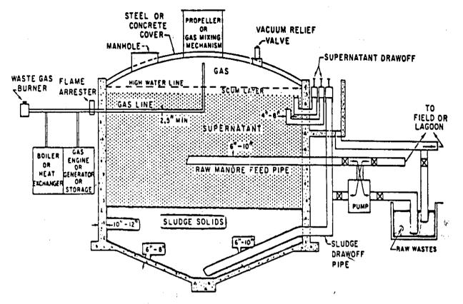
Figure 4. A Typical Fixed Wall Sewage Treatment Plant
