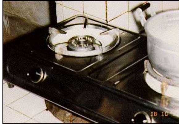
Biogas stove in China
