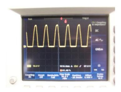
This is what the waveform will look like with no battery attached. It's a nice pulsed DC waveform. When a 12v battery is attached to the charger this spikes will go down to around 13-14 volts. This is a current limited charge, not a voltage limited charge. This means that the voltage will drop down to half a volt or so above battery terminal voltage. As stated above, the advantage to using a current limited charge is that you can charge about any voltage battery.
