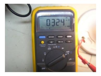
As you can see here, using a 60 watt light bulb, with the two charging terminals shorted together (NOT HOOKED UP TO THE BATTERY) the most current I will draw is 324mA or 1/3 of an amp. If you want less, use a smaller bulb. If you want more, go for a larger bulb. The bulb is the current limiter.
