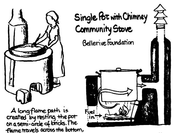
toward the front, and around the sides of the pot before reaching the chimney.
