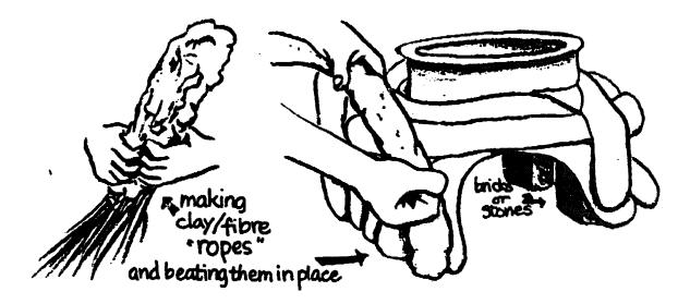
Fig. 21 Moulded stoves are (more often) accurately made, and can be transported if they have a significant fibre content.
