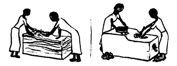
Fig. 20 'Ropes' of 50% clay/50% long fibres (either hay or raw sisal) are prepared, then interlocked and beaten into place around pots resting on three stones or bricks.
