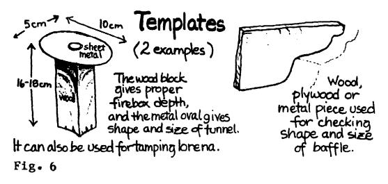
The use of moulds or templates in the production process increases the confidence of the trainee and uniformity of the stoves, and decreases the time required to train the builders and to construct the stoves.
