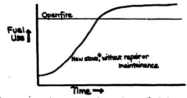
"Actual curve depends on type of store. Repairs will also significantly alter the curve. Based on information gained in Indonesia. by ITDG.
