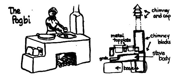
One person can produce a moulded stove in half a day, and a two pot-hole carved stove in one or two days. The total time taken depends on whether a chimney is installed and how much time
