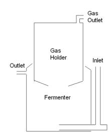
The feedstock must be blended so that it is smooth using a blender powered by electricity or by hand. Two kilograms of such feedstock Figure 3: Compact biogas digester
