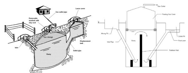
Figure 1: Fixed dome digester
