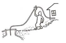
b). When the pipeline is not buried under the soil, you could lift the pipeline towards the digester and let the water fall back into the digester.
