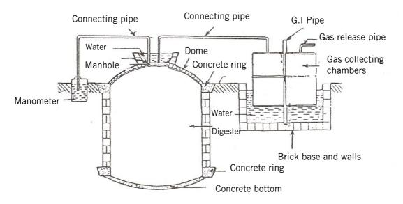
The special advantages of the Sri Lankan bio-digester
