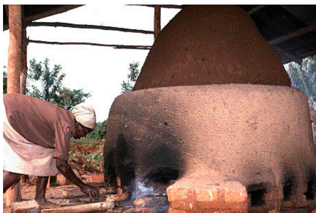
Figure 3: Charcoal Kiln, Kenya. Photo: Heinz Muller / Practical Action.
