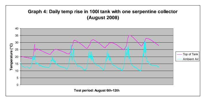
Table 4: August and November tests: daily temp. rise in the tank in a 100I tank with one collector.
