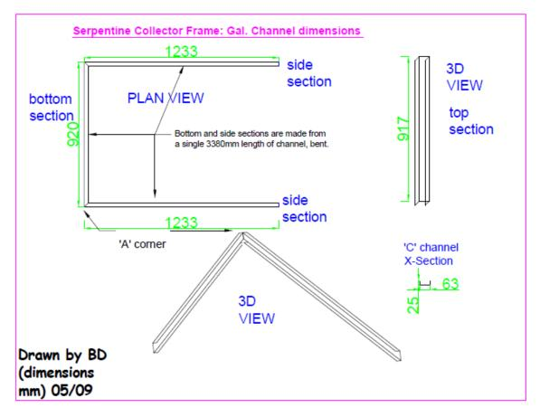
The absorber size determines the dimensions of the frame.
