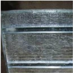
Collector frame mounted to insulated backing plate with spacers
