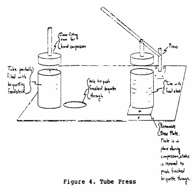
and a close fitting ram used for compaction. The basic design can be varied considerably, as the figure indicates.
