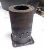
air inlet. The top of the tube has cast iron fins to swirl the flame. I think a ten inch length of four inch black pipe would work just as well if you do not have access to a burner tube like this.
