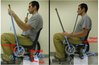
a. LFC in low gear b. LFC in high gear Figure 3. Changing mechanical advantage by moving hand position on the levers
