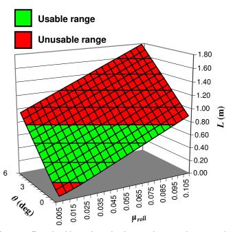
Figure 4. Required lever lengths for varying terrains at peak efficiency power output
