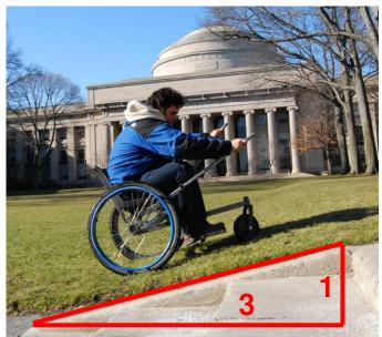
Figure 11. LFC going up 1:3 rise during hill climb trials
