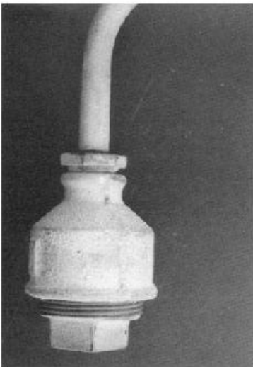
Figure 4: Components of the assembled mercury retort
