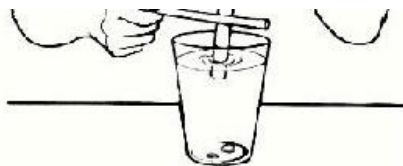
Figure 6: Tap the pipe to remove the mercury
