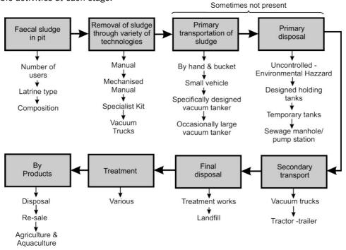
Figure 1: The FSM process, from generation to by-products [Illustrator: Niall Boot 2007]
