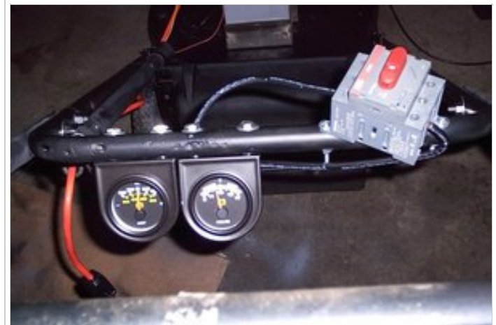
Ammeter and Voltmeter
