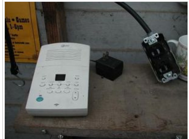
Fig.16 To test the draining abilities of the battery, the 4 watt answering machine as a test load
