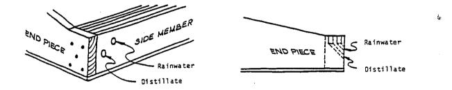
Drill two holes as shown in both sides. Door end only.
