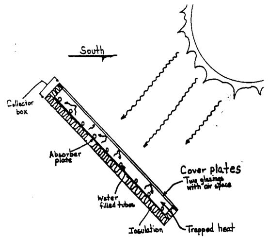
Figure 1. Solar Absorber
