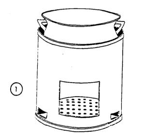
Figure 2. Wedge-shaped pot support made from scrap sheet metal.
