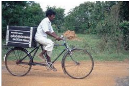
Figure 3: Extended bicycle Photo: Practical Action
