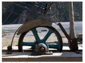
A typical braking system
