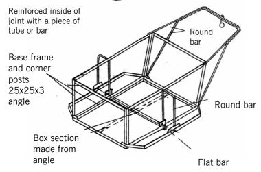
Figure 6 shows a frame that can be made from angle and bar
