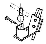
Figure 7: Hitch design. A stee or rubber ball drops into a socket formed from flat bar or cut from a pipe bolted to the carrier or frame of the bicycle
