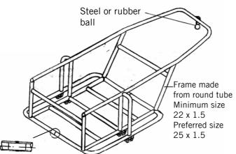
Alternative frame constructions can be used depending on materials and the production equipment available.
