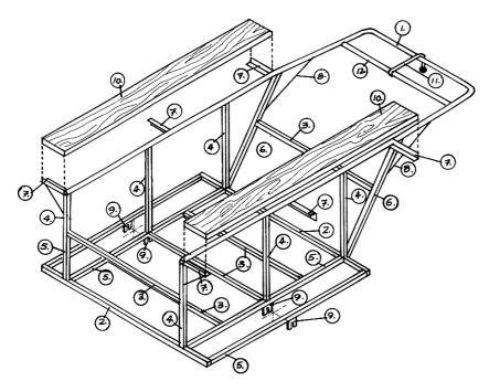
Figure 4: The frame construction is made up from welded steel tube
