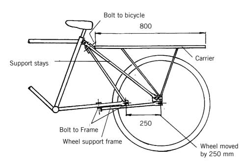
Figure 4: Construction of extension for a standard bicycle
