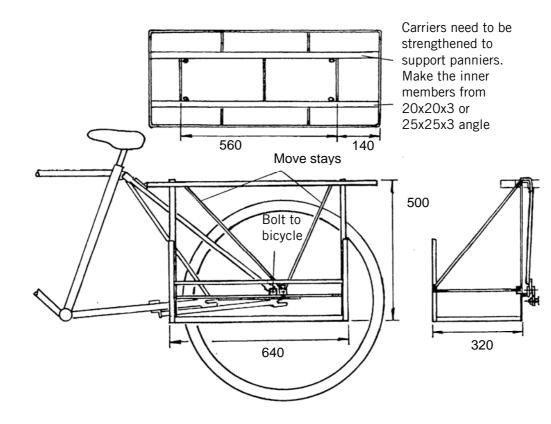
Figure 2: Construction of panniers
