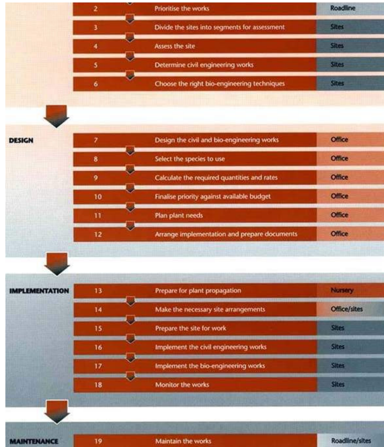
Figure 1.3: Flow chart to show the progression of the steps for slope stabilisation
