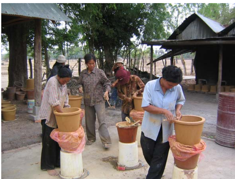
Putting finishing touches on the filter elements before firing in the kilns
