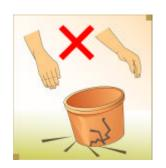
If a ceramic pot full of water takes less than 3 hours to empty, the flow rate is too fast and the ceramic pot should be replaced.
