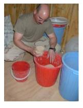
The dry mix should be mixed thoroughly in a container, cement mixer (for larger batches), or a plastic sheet on the floor rolled back and forth. Remember that every time we increase the amount of clay to the mix we decrease the final flow rate of the filter. It is crucial to experiment with the percentage to obtain the optimal proportions by volume.
