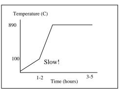
escape before it boils at 212°F. After 212°F the temperature can be raise quickly to 1650°F (890°C) and held there for several hours to cook the pot. After the pot is cooked, the kiln can be allowed to cool slowly over 2 hours until the pot can be handled by hand. Careful not to damage the pot while it is hot.
