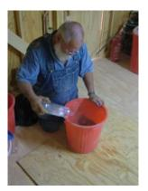
little drier than a typical cement mix. Just when the clay begins to hold its shape when squeezed out through the hands it is ready. If it is too wet it will slump in the press or fall over when drying.
