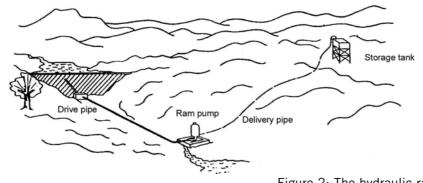
Figure 2: The hydraulic ram pump system
