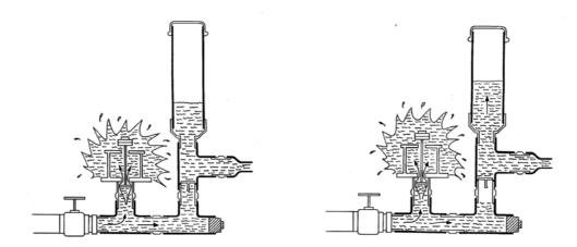
Figure 1: The hydraulic ram pump
