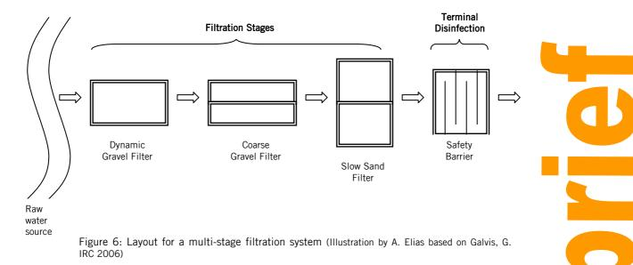
This system combines some of the less complex processes of water treatment: coarse gravel filtration and slow sand filtration. Removing large particulates through sedimentation or sand traps should still be carried out before running water through a multi-filtration system. It is most suited to rural communities and small to medium sized towns where the use of chemical treatment or more complex technologies would not be feasible.
