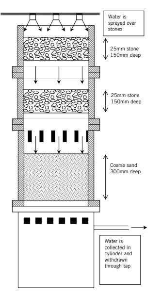
Figure 2: A cylinder aeration system. (Illustration by A. Elias based on Pickford (1977))
