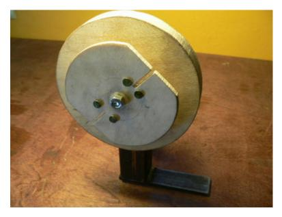
Put the front on and use the wing nut to hold it on there. (Ours which is featured in the pictures uses a normal nut - a wing nut is easier though) The coil winder is finished, we'll discuss how to use it when we start making the stator.
