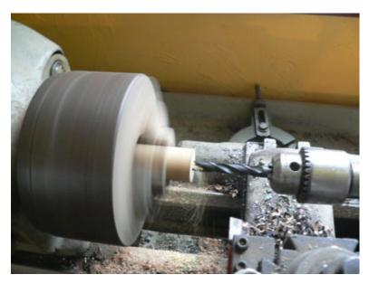
We cut the dowel off with any saw, and then drill it out on the lathe. While it's on the lathe it's nice to round the edges and sand it a bit. If you don't have a lathe, you could do this carefully with a hand drill or drill press, or - if it's just for one machine the wooden handle is not very important, it just makes for more comfortable winding.
