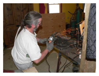
Whenever we cut metal there are sharp burrs at the cut. It's nice to cleanup all our cuts (and welds) with a grinder. Pictured above George is grinding the cuts (he should be wearing a face mask).
