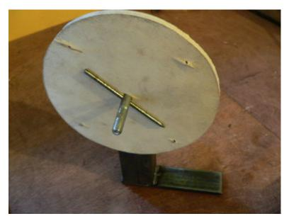
Insert the pin through the shaft and center it.
