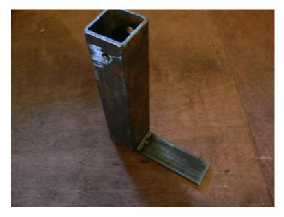
Weld the 5" long bar stock that has no holes in it to the bottom (the end furthest from the hole) of the square tubing. This serves as a base so that we can clamp the coil winder to a workbench.
