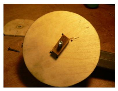
Put the small rectangular spacer on and align it so that its in between all the 4 holes which will hold the pins around which the coil is formed. Tack it there with a touch of glue so it doesn't rotate.
