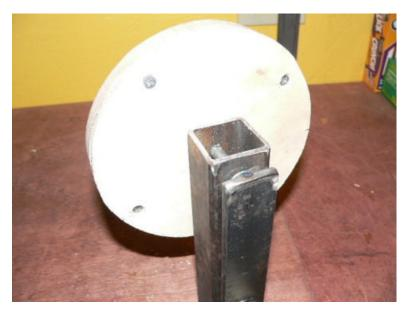
Use 5/8" long wood screws to screw the two disks together coming in through the back of the coil winder, through the 4 holes we drilled and countersunk earlier. The screw heads need to be flush, they must not stick out.
