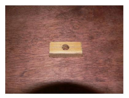
Cut a piece of 3/8" plywood rectangular as shown above. It's 1.5" tall, and 3/4" wide. Drill a 5/16" hole through the center. This serves as a spacer between the disks.
