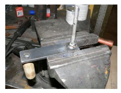
Take the longer bolt (the one with the hole drilled in it) and weld it to the other end of the handle as shown in the picture. It needs to be square !
