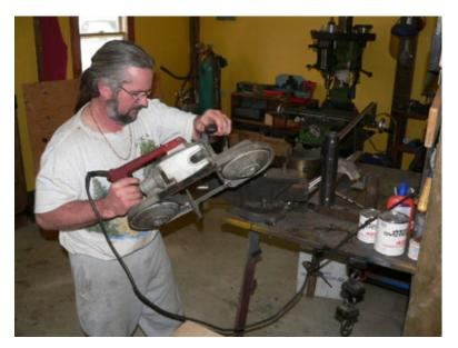
First step is to cutout some metal parts. I find the portable metal cutting band saw fast and easy, but a hack saw, saw zall or even a torch would work fine. In building wind turbines we often have to adapt a design to accommodate the tools are resources that are available to us, sometimes this requires some imagination.
