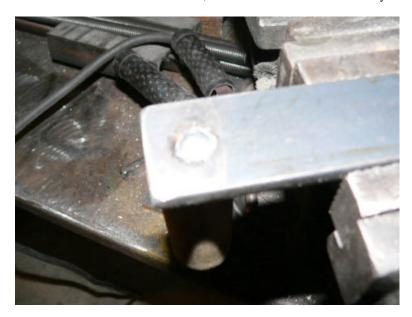
Turn it over and spot weld where the bolt is through the bar stock -this assures that the handle will never come loose.
