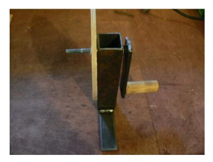
Put another washer on and then put the 6" diameter 1/4" thick disk on. The countersunk holes need to be pointing back, towards the handle.
