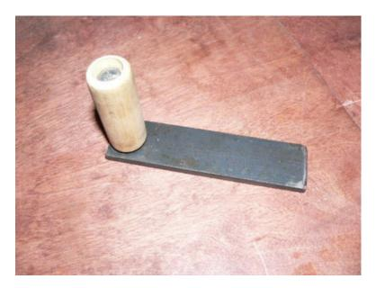
Put the shorter bolt (2.5" long) through the wooden handle and thread it into the 5" long bar stock which has been drilled and tapped to accept the bolt. Put a washer in between the handle and the bar stock. Thread the bolt in so that the threads come flush with the back of the bar stock, and the handle should turn freely.
