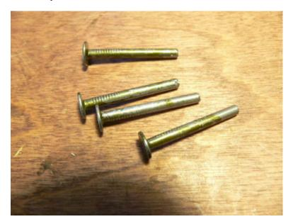
Cut 4 16 penny nails and cut them 1.125" long (including the head). De-burr the ends you've cut (so they're not sharp). Once the coil winder is finished, we'll insert these through the 4 holes in the front (4" diameter) disk and they'll also go into the holes in the rear disk, so that the disks are pinned together and the pins will be supported both in the front and in the back. These 4 pins will form the center of the coil.
