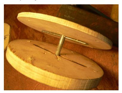
Put the 5/8" thick disk on the shaft so that it fits over the pin that's through the shaft, and bring it tightly against the  $\frac{1}{4}$ " thick disk.
