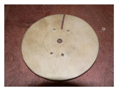
Cut a slot in the front 4" diameter disk as shown. It should be about 1/8" wide and should come right to the center, and stop between the two pins that are nearest each other. We'll start winding the coils from this slot and it needs to be centered at the narrowest part of the coil.
