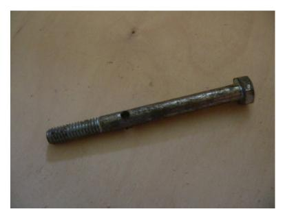
Drill a hole (9/64") through the 3.5" long bolt. The hole should be drilled on center at 2 3/8" from the bottom of the bolts head. The 9/64" hole is a good diameter to fit a 16D nail pretty tightly.
