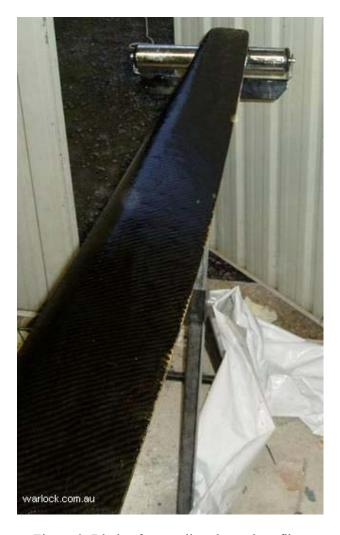
Figure 9. Blade after sanding the carbon fibre
