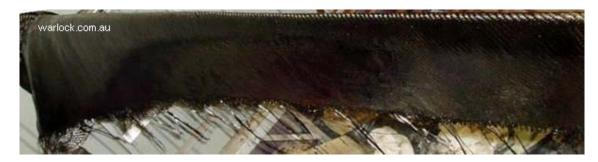
Figure 8. Blade after being covered in uni-directional carbon fibre
