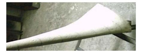
Figure 5. Polyurethane foam blade after sanding
