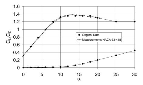
*Figure 2-28 Original airfoil characteristics for t/c=18% on the LM 19.1 blade.*
