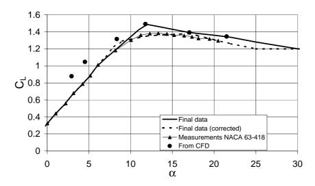
Figure 2-17 Constructed  $C_L$  at r=12.5 m corresponding to 18.20 % thickness. Comparison with 2D wind tunnel measurements.
