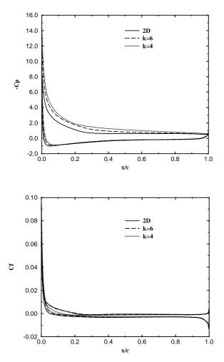
Figure 4-4  $C_p$  and  $C_f$  distributions on a NACA 63<sub>2</sub>-415 airfoil at incidence 20° and  $Re=1.5 \times 10^6$ .
