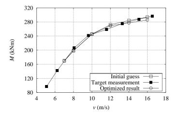
Figure 3-17 Blade root flapwise bending moment at r = 0.8 m for optimised result compared with initial guess and target measurements.
