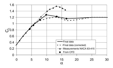
Figure 2-21 Constructed  $C_L$  at r=19.0 m corresponding to 15.75 % thickness. Comparison with 2D wind tunnel measurements.
