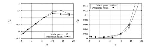
Figure 3-2  $C_L$  and  $C_D$  at t/c = 16.5% at r = 16.5 m corresponding to NACA 63-216.5 for optimised result compared with initial guess.
