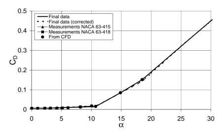
Figure 2-20 Constructed  $C_D$  at r=16.5 m corresponding to 16.55 % thickness. Comparison with 2D wind tunnel measurements.
