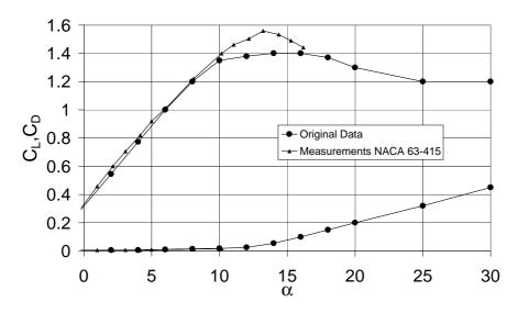
*Figure 2-27 Original airfoil characteristics for t/c=15% on the LM 19.1 blade.*
