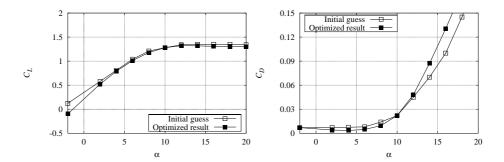
Figure 3-13  $C_L$  and  $C_D$  at t/c = 18% at r = 13.9 m corresponding to LM2-18 for optimised result compared with initial guess.
