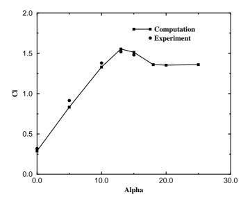
Figure 4-2 Comparison of computed 2D  $C_L$ -coefficient vs.  $\alpha$  of a NACA 63<sub>2</sub>-415 airfoil at Re=1.5×10<sup>6</sup> with experimental data at Re=3×10<sup>6</sup>.
