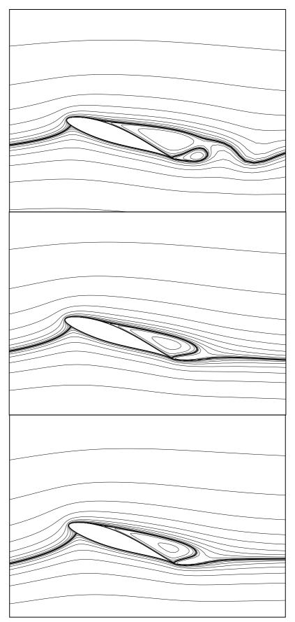
Figure 4-3 Stream lines for the flow around a NACA  $63_2$ -415 airfoil at incidence 20° and Re=1.5x10<sup>6</sup>, (a) 2D, (b) k=6, (c) k=4.
