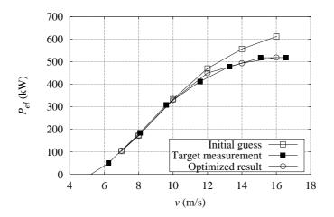
*Figure 3-16 Electric power for optimised result compared with initial guess and target measurements.*
