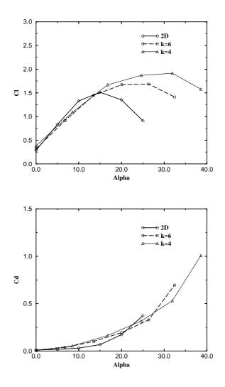
Figure 4-5  $C_L$  and  $C_D$  vs.  $\alpha$  of a NACA 63<sub>2</sub>-415 airfoil at Re=1.5x10<sup>6</sup>.
