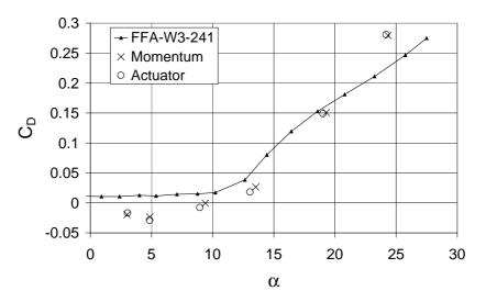
Figure 2-8 Derived  $C_D$  at r=10.0 m (t/c=24.19%) using momentum theory and actuator disc theory. Comparison with 2D wind tunnel measurements.
