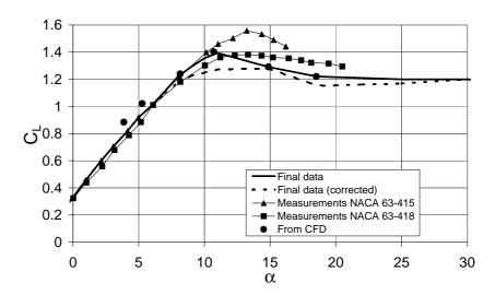
Figure 2-19 Constructed  $C_L$  at r=16.5 m corresponding to 16.55 % thickness. Comparison with 2D wind tunnel measurements.
