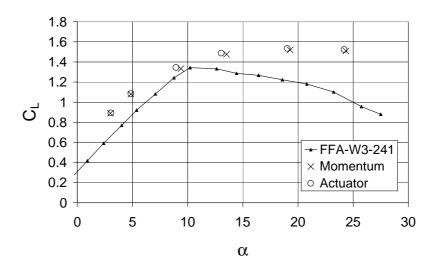
Figure 2-7 Derived  $C_L$  at r=10.0 m (t/c=24.19%) using momentum theory and actuator disc theory. Comparison with 2D wind tunnel measurements.
