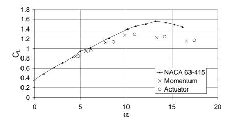
Figure 2-11 Derived  $C_L$  at r=19.0 m (t/c=15.75%) using momentum theory and actuator disc theory. Comparison with 2D wind tunnel measurements.
