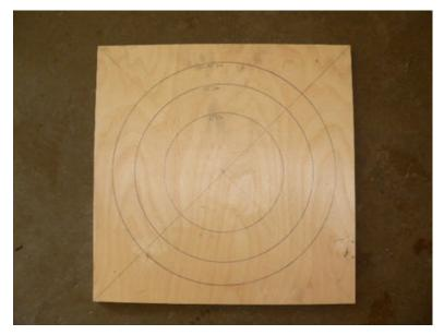
Find the center of the square. (an easy way is to draw light lines from corner to corner - where they intersect is center).
