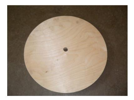
Cut out another disk from birch plywood, 16" diameter. This is the lid for the mold. Sand the edges smooth. Drill a 3/4" diameter hole in the center and give it a slight taper with a round file. (sand paper wrapped around a wooden dowel or bolt works nicely too)
