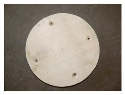
Cut out another disk 5.75" in diameter. This will be the island in the center of the mold. It also needs to be sanded smooth and slightly tapered. Drill 4 holes for wood screws as shown in the picture and run the countersink in just like you did for the middle part of the mold.
