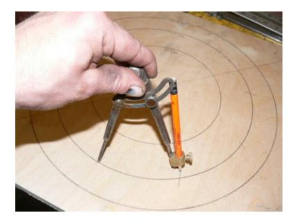
Use dial calipers to adjust your compass as shown in the picture. Then pick a starting point on the 12" circle and use the compass to divide the circle into 9 equal parts. This is a nice way to divide any circle - it's very handy for placing magnets and coils accurately in different sized wind turbines.
