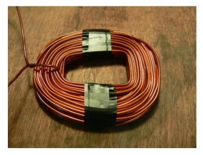
We refer the longest sides of the coil as the 'legs'. Tape the legs of the coils with a couple wraps of electrical tape to hold things together. One coil is finished.
