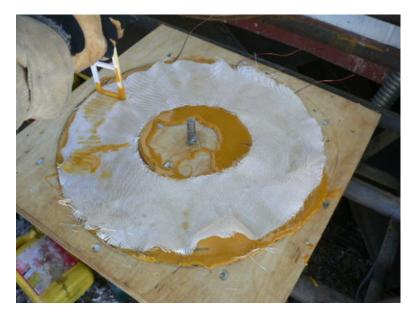
Put the remaining fiberglass ring over the top of the coils and work resin into it - again, it should almost disappear.
