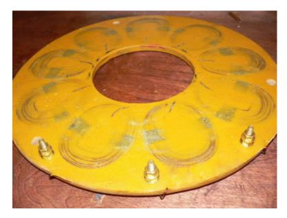
The stator is finished! We can put that aside untill we're ready to assemble the alternator.
