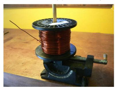
Start by creating some kind of fixture to hold the spool of magnet wire. I usually use a vice with a piece of threaded rod, or a wooden dowel sticking up to put the spool. Clamp it to the work bench securely.
