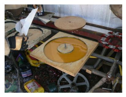
It takes about exactly 1/2 gallon of resin to cast the stator. Find a level place to put the mold. It's important to either keep the edges of the mold off the workbench - or find a work bench (like the one in the picture) that allows access for C clamps around the edges of the mold. When your done you'll need to clamp the lid down with C clamps so think ahead! Pour about a pint of resin into the mold and roll the mold around so that the whole bottom and the sides become covered 'wet' with resin.
