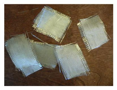
Cut 9 little rectangles from fiberglass cloth about 1.5" wide and 2" long. Before you cast the stator you'll need to remove the coils from the mold again. We'll use these squares of cloth and superglue to hold everything together so that we can move it.
