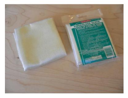
The stator will be cast in the same polyester resin you used for the magnet rotors. You'll need fiberglass cloth on both sides of the coils. It might be useful to reveiw the section on casting magnet rotors before doing this as the proceedure is very similar and safety precautions are the same.
