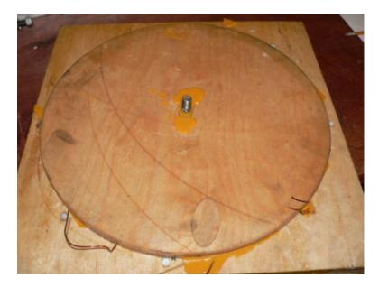
Once the resin seems hard then remove the C clamps and the nut in the center. Use a chisel or a screw driver to gently pry around the lid untill it breaks loose.
