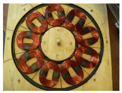
Once all three phase are finished, put all three back into the mold as shown in the picture. Do it such that your three 'ends' (those wires that are pointing towards the outside of the mold) are beside each other. Those three 'ends' will be the leads out of the stator (the output from the wind turbine).
