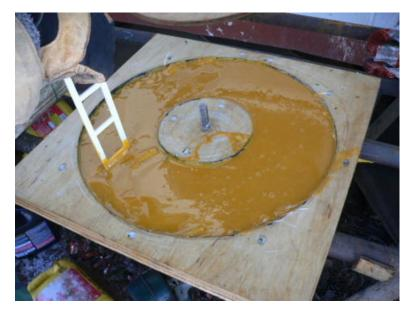
Then pour about another pint of resin in the mold, work it into the fabric more - try to work out any airbubbles.
