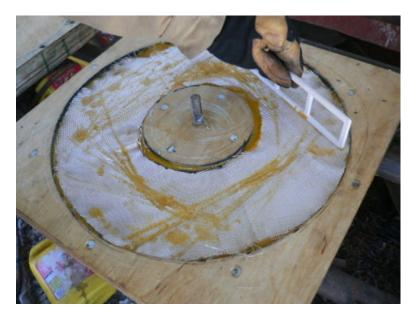
Put one of the fiberglass rings into the resin and work it with a stick untill it becomes saturated. When saturated - the fabric will become almost invisible. (you won't see any white)
