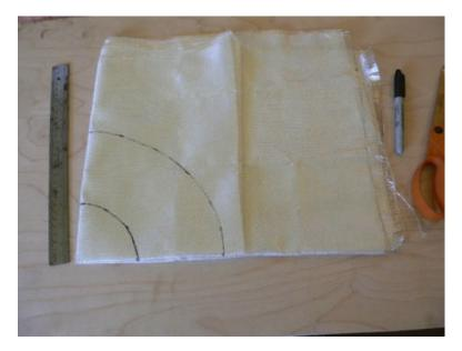
If you fold the fabric correctly, you can lay out just 1/4 of the ring and cut out two in one shot. You need two rings of fiberglass 15" outer diameter and 6" inner diameter.
