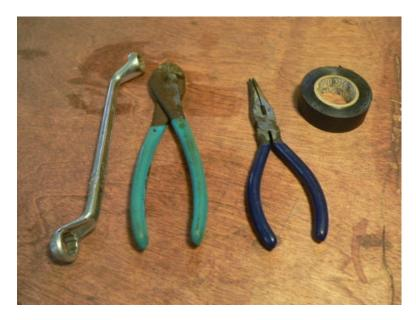
You'll need a pair of side cutters (to cut the wire), a pair of needle nosed pliers (to bend the wire) and some electrical tape. If the coil winder has a wing nut holding it together then you can use your fingers to take it apart. Otherwise you'll need a 1/2 wrench. When you bolt the front on the coil winder finger tight is fine, but after all the wire is wound on the spool the nut will be tight so - if you dont have a wing nut, you'll need a wrench to get it apart.
