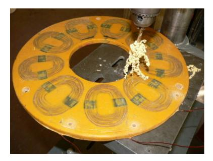
Drill 3 holes 1/4" in diameter about 1/2" away from the edge of the stator - one near each of the leads that's coming out.
