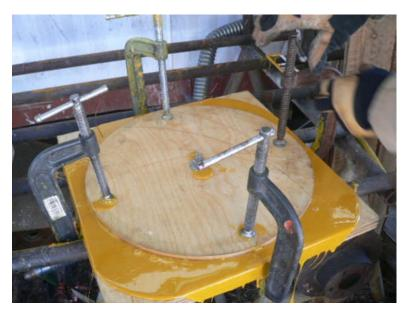
Put a C clamp on each side of the mold (use 4 C clamps) and tighten them evenly. You'll have some idea when the resin is hard by all the stuff that spilled out the side! Let the stator sit in the mold untill the resin is hard.
