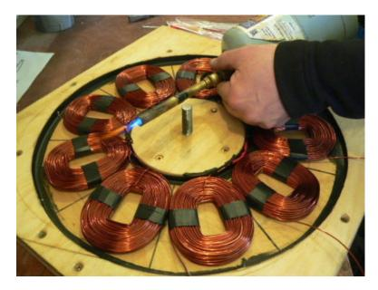
Now you need to make the star connection between the phases. The 3 inside leads should be brought together so that we can connect them together. Leave enough slack in the wires so that we can make this connection, and then push it down between the coils and the island in the mold. So figure the length, cut them off, burn the insulation with the torch, sand it, twist them and solder them. Then insulate the connection with electrical tape or heat shrink.
