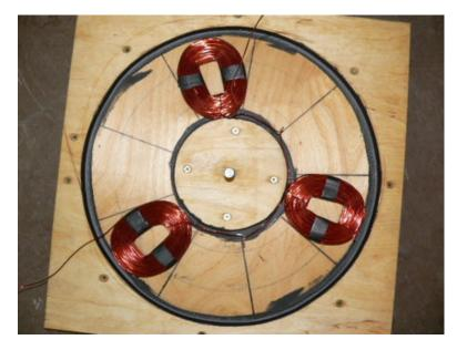
Put the 3 coils back in the mold and twist the wires together tightly. You can see in the picture how the connections are pretty much centered in between the coils. Then solder the connections, and bend them over with pliers so you can insulate them with electrical tape and keep it all as thin as possible. You can also use heat shrink here for neater appearance - if you do, be sure to put that on before you twist the leads together!
