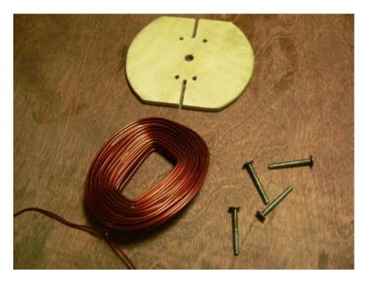
The coil should pretty much fall off the end if you just turn it over. Do it carefully so the coil doesn't fall apart.
