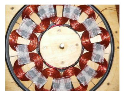
Remove the duct tape, it should pull off easily.
