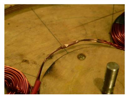
If you're building a 12 Volt machine with multiple strands of wire it can be tricky to twist things together nicely. For machines that have multiple strands, it works well to make your connections by inserting the coil leads into small copper, or brass tubing - and then crimp and solder.
