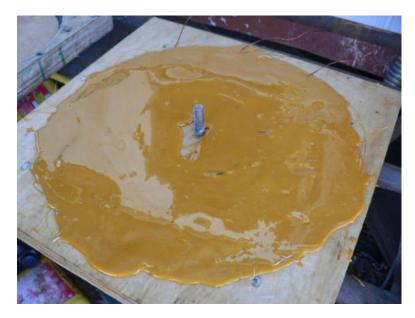
Pour the remaining resin over the top of the fabric. Work it in and try to work out air bubbles. It might not hurt at this time to beat on the mold a bit or vibrate it with a sander (or something) for a couple minutes to help air bubbles rise to the top.
