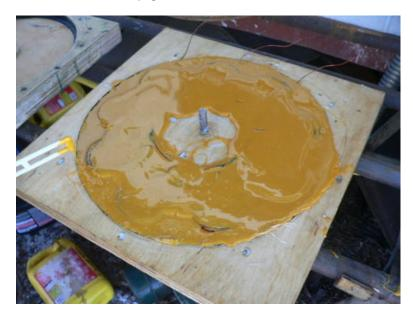
Then fill the mold with resin and be sure all surfaces of the coils have resin on them.
