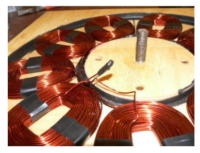
Pictured above is the finished star connection, all that needs to be done is to poke it down so it doesn't stick up above the coils.
