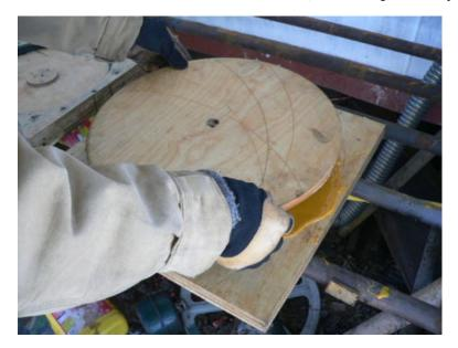
Carefully put the lid of the mold down over the casting.
