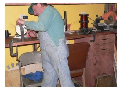
Pictured above Scott's winding with two strands of wire. This is necessary for 12 Volt machines.
