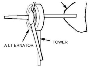
The wind generator is suitable for family needs such as lighting and radio, powered by a 12-volt battery. It is for low and medium windspeeds, common in Peru and Sri Lanka, where the wind turbine is being built.
