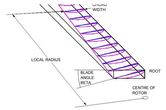
At the root, the shape of the blade changes from an airfoil section into a shape which is suitable for the hub assembly
