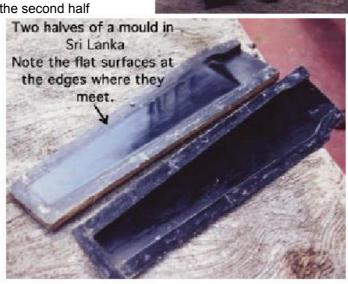
flat surface, so that the two moulds fit each other perfectly.
