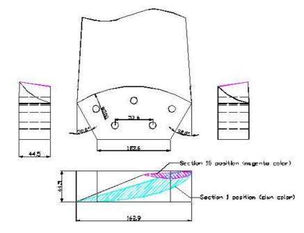
The blade root needs to be shaped to mount easily onto the wind generator. In Peru the root shape is as shown above. All three blade roots are clamped between two steel plates. The transition between the root (mounting portion) and the blade (airfoil
