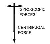
If there is a problem with inadequate strength in the blades, then increase the amount of fibreglass, especially in the root area. The resin has no real strength except to bond the glass fibres. If possible, use uni-directional fibreglass mat. It may not be easy to find, but it is has double the tensile strength for the same weight. This is a big advantage where the main forces are inertial (centrifugal, and gyroscopic).
