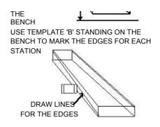
station. When the pattern is finished, the top edge of the template should be exactly level, and the leading and trailing edge lines should meet the lines drawn earlier on the sides of the workpiece.
