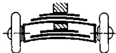
i) wheel suspension by means of cross springs
