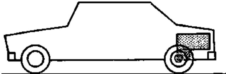
Figure 1/3 Rear-axle drive (rear-mounted engine)
