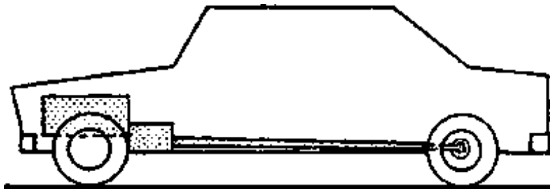
Figure 1/1 Rear-axle drive (front-mounted engine)
