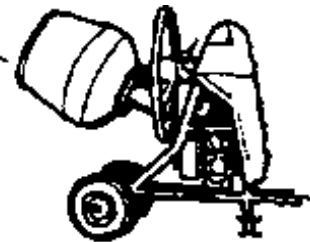
C Small hand-fed tilting drum mixer
