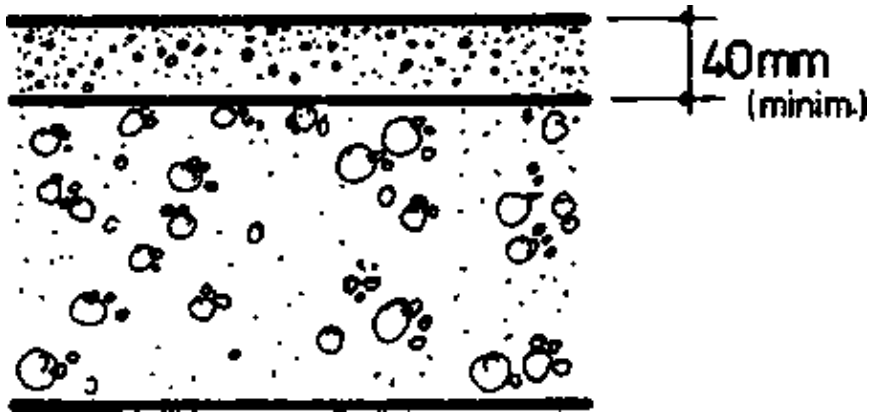
7.511b SEPERATE CONSTRUCTION
