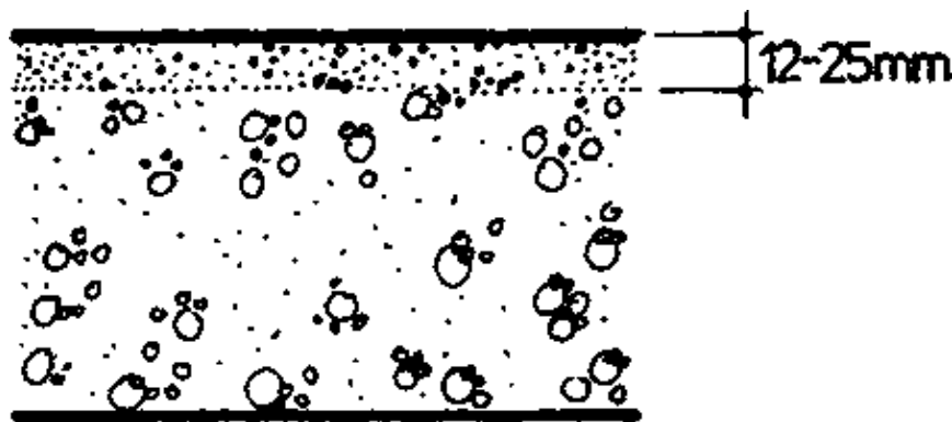
7.511a MONOLITHIC CONSTRUCTION
