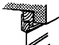
10 Easy removal of door at 90° or 180° (Continental type hinge)
