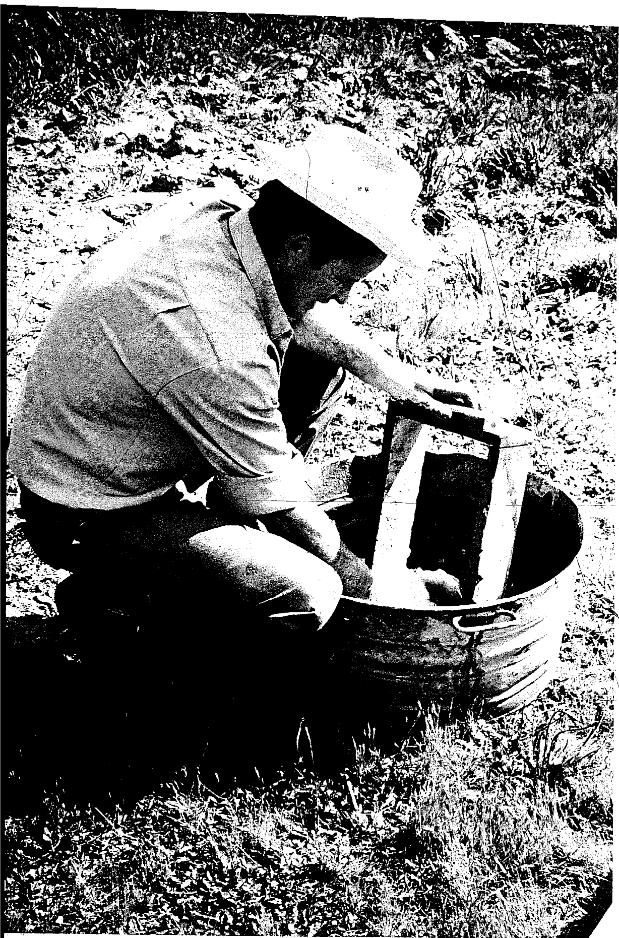
Washing the mold. If you don't, the corners of the next brick will tear off on mud left from the last one.
