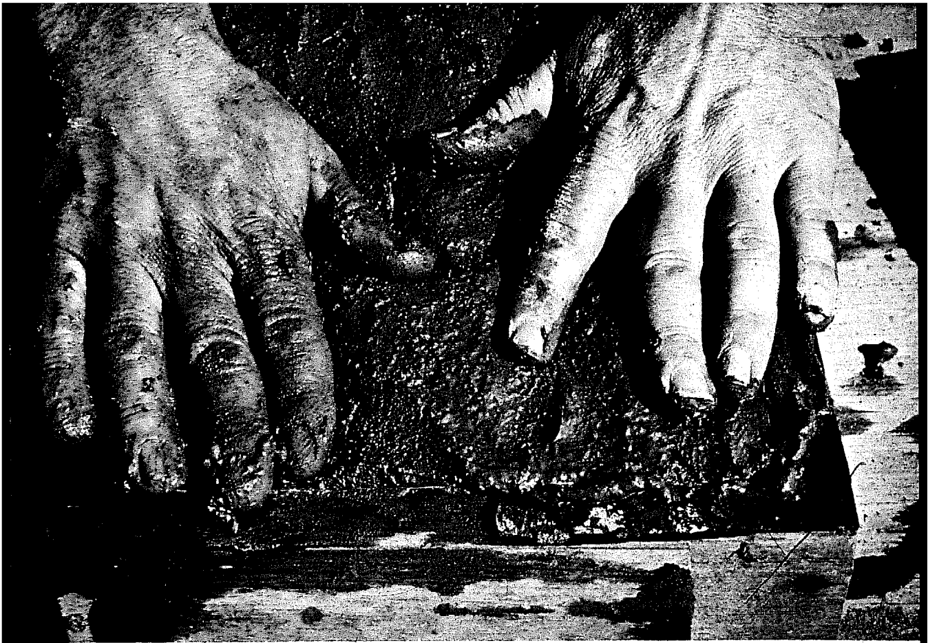
Working the mud into the corners of the mold. You can see the iron corner brace screwed to the mold.
