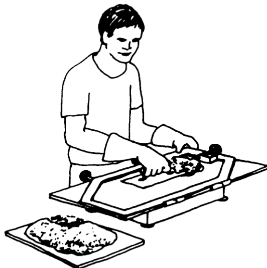
Figure 2: Work the mortar mix under vibration
